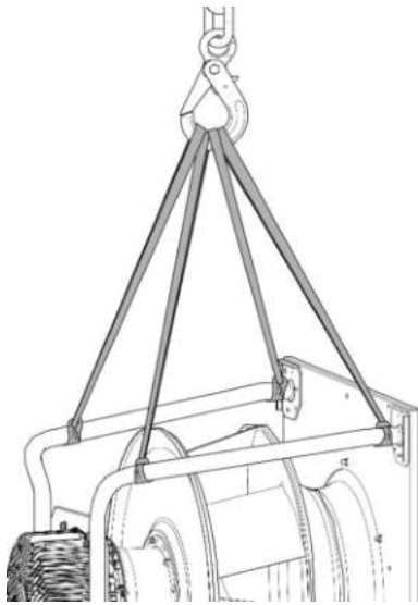
Fig. 1: Hoisting diagram for transportation of RadiPac
