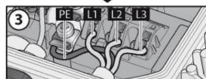
Fig. 2: Connecting wires to terminals
