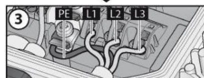
Fig. 2: Connecting wires to terminals
