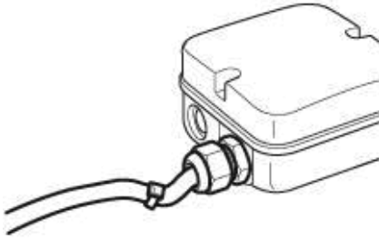
Fig. 1: Fan installed lying flat, cable routed in a U-shaped loop.
