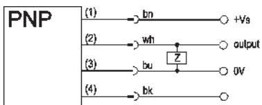
The alternating current devices are usually 2-wire devices without short-circuit protection. Consequently a load must be connected, which allows for a minimum load current of 2mA, however, not exceeding the maximum load current.
