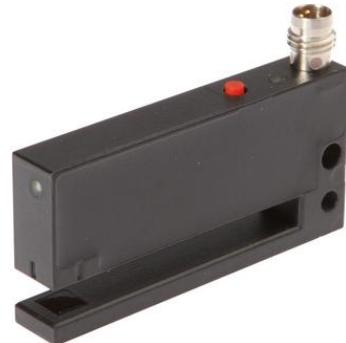
Special design of through-beam sensor. Transmitter and receiver are located in the fork or angular limbs and are perfectly aligned to each other.
