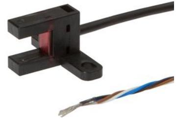
Special design of through-beam sensor. Transmitter and receiver are located in the fork or angular limbs and are perfectly aligned to each other.
