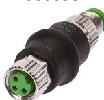
Adaption, M8 Female (socket) 3pin Straight, M8 Male (connector) 4pin Straight, 24V, -25-85°C, IP67, Oil and cooling lubricants, Welding area
