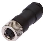
Cable socket, Straight, Suitable for self-assembly, Soldering connection, Ø3.5-5mm, 4A, 60V, -40-85°C, M8 Female (socket) 3pin, IP67, Brass
