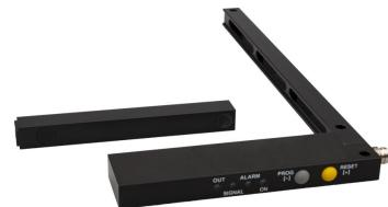
Special design of through-beam sensor. Transmitter and receiver are located in the fork or angular limbs and are perfectly aligned to each other.
