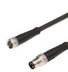
Connection cable, 0.3m, M8 socket 4-pin straight, M8 connector 4-pin straight, 4-core, PUR (polyurethane), suitable for trailing chain and torsion-resistant, oils and cooling lubricants, welding area, silicone-free
