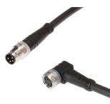
Connection cable, 0.3m, M8 socket 4-pin angular, M8 connector 4-pin straight, 4-core, PUR (polyurethane), suitable for trailing chain and torsion resistant, oils and cooling lubricants, welding area, silicone-free
