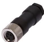
Cable socket, Straight, Suitable for self-assembly, Soldering connection, Ø3.5-5mm, 4A, 30V, -40-85°C, M8 Female (socket) 4pin, IP67, Brass
