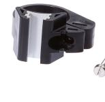
accessories magnetic, Mounting clip, 30x34x19mm, span 20.1-21. 8mm, Plastic, For sensor MZ07, for Cylinder, 20round
