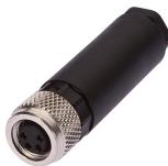
Cable socket, Straight, Suitable for self-assembly, Screw connection, Ø3.5-5mm, 4A, 30V, -40-85°C, M8 Female (socket) 4pin, IP67, Brass
