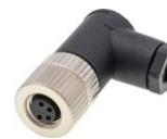
Cable socket, Angular, Suitable for self-assembly, Screw connection, Ø5mm, 4A, 60V, -40-85°C, M8 Female (socket) 4pin, IP67, Polyamide PA
