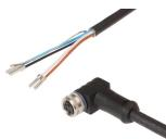
Connection cable, 5m, M8 Female (socket) 4pin Angular, Free conductor end, 4x0.34mm<sup>2</sup>, PUR (Polyurethane), Ø5.5mm, 60V, -25-90°C, IP67, Shielded, Suitable for trailing chain and torsion resistant, Oil and cooling lubricants, Welding area, Silicone..
