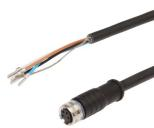
Connection cable, 5m, M8 Female (socket) 4pin Straight, Free conductor end, 4x0.34mm<sup>2</sup>, PUR (Polyurethane), Ø5.5mm, 60V, -25-90°C, IP67, Shielded, Suitable for trailing chain and torsion resistant, Oil and cooling lubricants, Welding area, Silicone..
