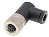
Cable socket, Angular, Suitable for self-assembly, Screw connection, Ø5mm, 4A, 60V, -40-85°C, M8 Female (socket) 4pin, IP67, Polyamide PA
