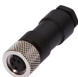
Cable socket, Straight, Suitable for self-assembly, Soldering connection, Ø3.5-5mm, 4A, 30V, -40-85°C, M8 Female (socket) 4pin, IP67, Brass
