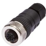
Cable socket, Straight, Suitable for self-assembly, Screw connection, Ø3-6.5mm, 4A, 240V, -25-90°C, M12 Female (socket) 4pin, IP67, PBT
