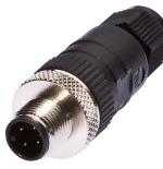
Cable connector, Straight, Suitable for self-assembly, Screw connection, Ø3-6.5mm, 4A, 240V, -25-90°C, M12 Male (connector) 4pin, IP67, PBT
