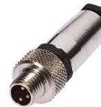
Cable connector, Straight, Suitable for self-assembly, Soldering connection, Ø3.5-5mm, 4A, 60V, -40-85°C, M8 Male (connector) 3pin, IP67, Brass
