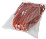
Plastic sheath, Ø17mm, Inner diameter 10mm, -40-250°C, Glass fiber with silicone rubber, Short-term resistance to weld spatter 1200°C, Tensile strength 400N, Flexible, Flame retardant, yard good
