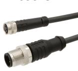
Connection cable, 0.3m, M8 socket 3-pin straight, M12 connector 3-pin straight, 3x0.34mm<sup>2</sup>, PUR (polyurethane), 60V, IP67, suitable for trailing chain and torsion resistant, oils and cooling lubricants, welding area, silicone-free
