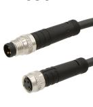
Connection cable, 0.3m, M8 socket 3-pin straight, M8 connector 3-pin straight, 3x0.34mm<sup>2</sup>, PUR (polyurethane), 60V, IP67, suitable for trailing chain and torsion resistant, oils and cooling lubricants, welding area, silicone-free
