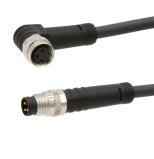
Connection cable, 0.3m, M8 socket 3-pin angular, M8 connector 3-pin straight, 3x0.34mm<sup>2</sup>, PUR (polyurethane), 60V, IP67, suitable for trailing chain and torsion resistant, oils and cooling lubricants, welding area, silicone-free
