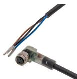
Connection cable, 5m, M8 Female (socket) 3pin Angular, Free conductor end 3pin, 3x0.34mm<sup>2</sup>, PUR (Polyurethane), Ø4.3mm, -30-90°C, IP67, With LED display, Suitable for trailing chain and torsion resistant, Oil and cooling lubricants, Welding area, S...
