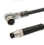
Connection cable, 0.6m, M8 socket 3-pin angular, M8 connector 3-pin straight, 3x0.34mm<sup>2</sup>, PUR (polyurethane), IP67, LED, suitable for trailing chain and torsion resistant, oils and cooling lubricants, welding area, silicone-free
