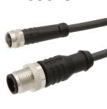
Connection cable, 0.3m, M8 socket 3-pin straight, M12 connector 3-pin straight, 3x0.34mm<sup>2</sup>, PUR (polyurethane), 60V, IP67, suitable for trailing chain and torsion resistant, oils and cooling lubricants, welding area, silicone-free
