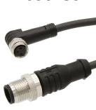
Connection cable, 0.3m, M8 socket 3-pin angular, M12 connector 3-pin straight, 3x0.34mm<sup>2</sup>, PUR (polyurethane), 60V, IP67, suitable for trailing chain and torsion resistant, oils and cooling lubricants, welding area, silicone-free
