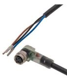
Connection cable, 2m, M8 Female (socket) 3pin Angular, Free conductor end, 3x0.34mm<sup>2</sup>, PUR (Polyurethane), Ø4.3mm, -30-90°C, IP67, With LED display, Suitable for trailing chain and torsion resistant, Oil and cooling lubricants, Welding area, Silicone...
