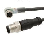
Connection cable, 0.3m, M8 socket 3-pin angular, M12 connector 3-pin straight, 3x0.34mm<sup>2</sup>, PUR (polyurethane), IP67, LED, suitable for trailing chain and torsion resistant, oils and cooling lubricants, welding area, silicone-free
