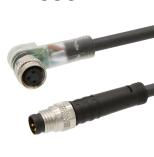
Connection cable, 0.3m, M8 socket 3-pin angular, M8 connector 3-pin straight, 3x0.34mm<sup>2</sup>, PUR (polyurethane), IP67, LED, suitable for trailing chain and torsion resistant, oils and cooling lubricants, welding area, silicone-free
