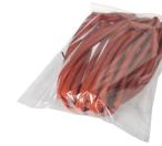
Plastic sheath, Ø17mm, Inner diameter 10mm, -40-250°C, Glass fiber with silicone rubber, Short-term resistance to weld spatter 1200°C, Tensile strength 400N, Flexible, Flame retardant, yard good
