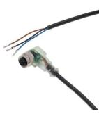
Connection cable, 2m, M12 Female (socket) 3pin Angular, Free conductor end, 3x0.34mm<sup>2</sup>, PUR (Polyurethane), Ø4.3mm, -30-90°C, IP67, With LED display, Suitable for trailing chain and torsion resistant, Oil and cooling lubricants, Welding area, Silic...
