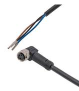
Connection cable, 2m, M8 Female (socket) 3pin Angular, Free conductor end, 3x0.34mm<sup>2</sup>, PUR (Polyurethane), Ø4.3mm, 60V, -40-90°C, IP67, TPU, Suitable for trailing chain and torsion resistant, Oil and cooling lubricants, Welding area, Silicone-free
