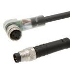
Connection cable, 0.3m, M8 socket 3-pin angular, M8 connector 3-pin straight, 3x0.34mm<sup>2</sup>, PUR (polyurethane), IP67, LED, suitable for trailing chain and torsion resistant, oils and cooling lubricants, welding area, silicone-free
