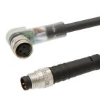
Connection cable, 0.6m, M8 socket 3-pin angular, M8 connector 3-pin straight, 3x0.34mm<sup>2</sup>, PUR (polyurethane), IP67, LED, suitable for trailing chain and torsion resistant, oils and cooling lubricants, welding area, silicone-free
