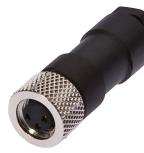
Cable socket, Straight, Suitable for self-assembly, Soldering connection, Ø3.5-5mm, 4A, 60V, -40-85°C, M8 Female (socket) 3pin, IP67, Brass
