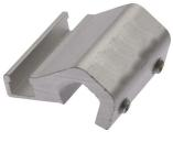
accessories magnetic, Mounting clip, 16x30x30mm, span 6.1-8. 5mm, Aluminum, For sensor MZ07, for Cylinder pull-rod, Screw mounting
