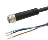
Connection cable, 2m, M8 female (socket) 3pin Straight, free conductor end, 3x0.34mm<sup>2</sup>, PUR (Polyurethane), Ø4.3mm, 60V, -30-90°C, IP67, suitable for trailing chain and torsion resistant, oil and cooling lubricants, welding area, Silicone-free
