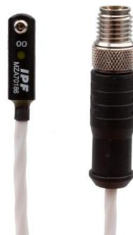
For many tasks in the field of automation technology, it is necessary to recognize the motional processes in pneumatic and hydraulic cylinders and to detect the position of the piston with precision. For this, magnetic cylinder sensors are used.
