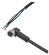
Connection cable, 2m, M8 Female (socket) 3pin Angular, Free conductor end, 3x0.34mm<sup>2</sup>, PUR (Polyurethane), Ø4.3mm, 60V, -40-90°C, IP67, TPU, Suitable for trailing chain and torsion resistant, Oil and cooling lubricants, Welding area, Silicone-free
