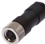
Cable socket, Straight, Suitable for self-assembly, Soldering connection, Ø3.5-5mm, 4A, 60V, -40-85°C, M8 Female (socket) 3pin, IP67, Brass
