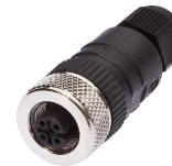
Cable socket, Straight, Suitable for self-assembly, Screw connection, Ø3-6.5mm, 4A, 240V, -25-90°C, M12 Female (socket) 4pin, IP67, PBT
