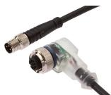
Connection cable, 0.6m, M12 socket 3-pin angular, M8 connector 3-pin straight, 3x0. 34mm<sup>2</sup>, PUR (polyurethane), IP67, LED, suitable for trailing chain and torsion resistant, oils and cooling lubricants, welding area, silicone-free
