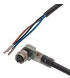
Connection cable, 5m, M8 Female (socket) 3pin Angular, Free conductor end 3pin, 3x0.34mm<sup>2</sup>, PUR (Polyurethane), Ø4.3mm, -30-90°C, IP67, With LED display, Suitable for trailing chain and torsion resistant, Oil and cooling lubricants, Welding area, S...
