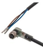
Connection cable, 2m, M8 Female (socket) 3pin Angular, Free conductor end, 3x0.34mm<sup>2</sup>, PUR (Polyurethane), Ø4.3mm, -30-90°C, IP67, With LED display, Suitable for trailing chain and torsion resistant, Oil and cooling lubricants, Welding area, Silico...
