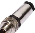
Cable connector, Straight, Suitable for self-assembly, Soldering connection, Ø3.5-5mm, 4A, 60V, -40-85°C, M8 Male (connector) 3pin, IP67, Brass
