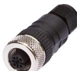
Cable socket, Straight, Suitable for self-assembly, Screw connection, Ø3-6.5mm, 4A, 240V, -25-90°C, M12 Female (socket) 4pin, IP67, PBT
