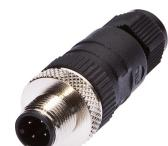
Cable connector, Straight, Suitable for self-assembly, Screw connection, Ø3-6.5mm, 4A, 240V, -25-90°C, M12 Male (connector) 4pin, IP67, PBT
