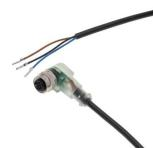
Connection cable, 2m, M12 Female (socket) 3pin Angular, Free conductor end, 3x0.34mm<sup>2</sup>, PUR (Polyurethane), Ø4.3mm, -30-90°C, IP67, With LED display, Suitable for trailing chain and torsion resistant, Oil and cooling lubricants, Welding area, Silic...
