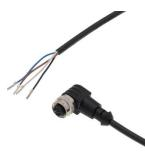
Connection cable, 2m, M12 Female (socket) 4pin Angular, Free conductor end, 4x0.34mm², PUR (Polyurethane), Ø4.7mm, 250V, -40-90°C, IP67, Suitable for trailing chain and torsion resistant, Oil and cooling lubricants, Welding area, Silicone-free
