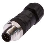
Cable connector, Straight, Suitable for self-assembly, Screw connection, Ø3-6.5mm, 2A, 30V, -25-85°C, M12 Male (connector) 8pin, IP67, PBT
