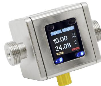
If an electrically conductive liquid moves across a magnetic field, a voltage is generated vertically to this magnetic field which is dependent on the flow velocity. This voltage is measured by electrodes located in the wall of the measuring tube. Microcontrollers evaluate this voltage, calculate the flow rate and show it on the display. An analog signal and a transistor switching output are available for further processing.
