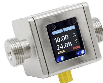
If an electrically conductive liquid moves across a magnetic field, a voltage is generated vertically to this magnetic field which is dependent on the flow velocity. This voltage is measured by electrodes located in the wall of the measuring tube. Microcontrollers evaluate this voltage, calculate the flow rate and show it on the display. An analog signal and a transistor switching output are available for further processing.
