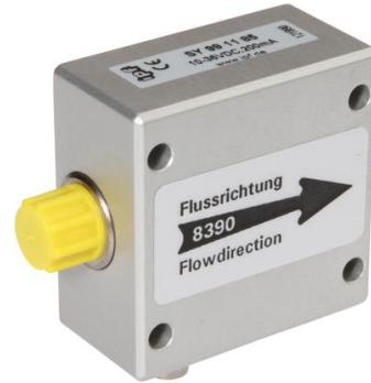
Flow sensor, lubricant, 23x63x45mm, hose AD 6mm, 10-36V DC, PNP NO, M8 connector, aluminum, pressure resistance 70bar
