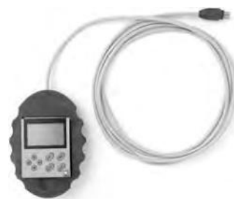
Diagnosis terminal with keypad and connection cable
