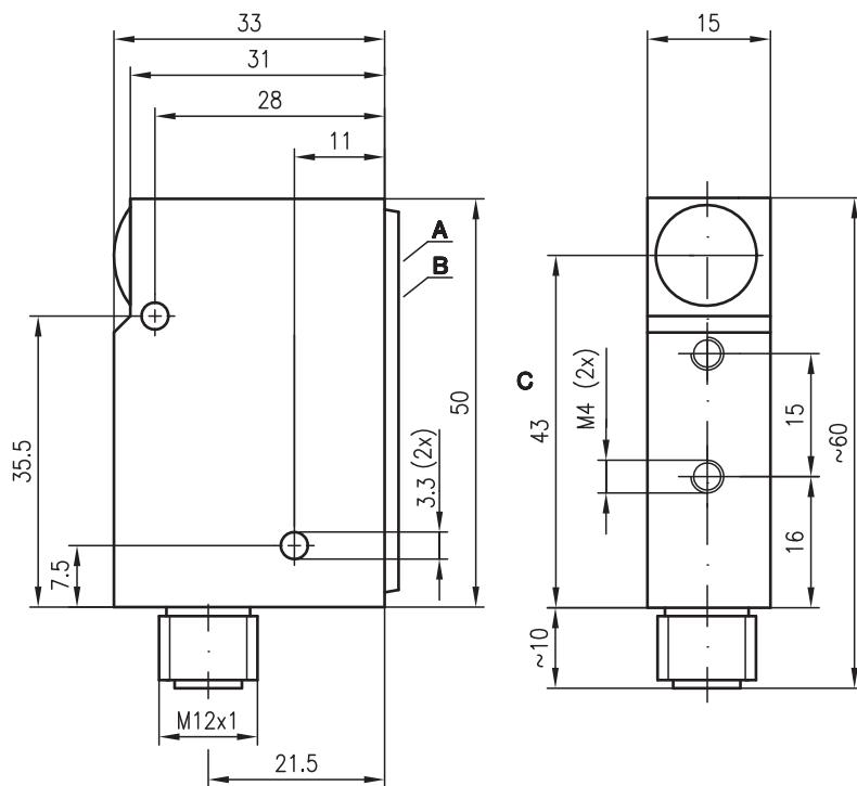
**A** Step switch for object adjustment
