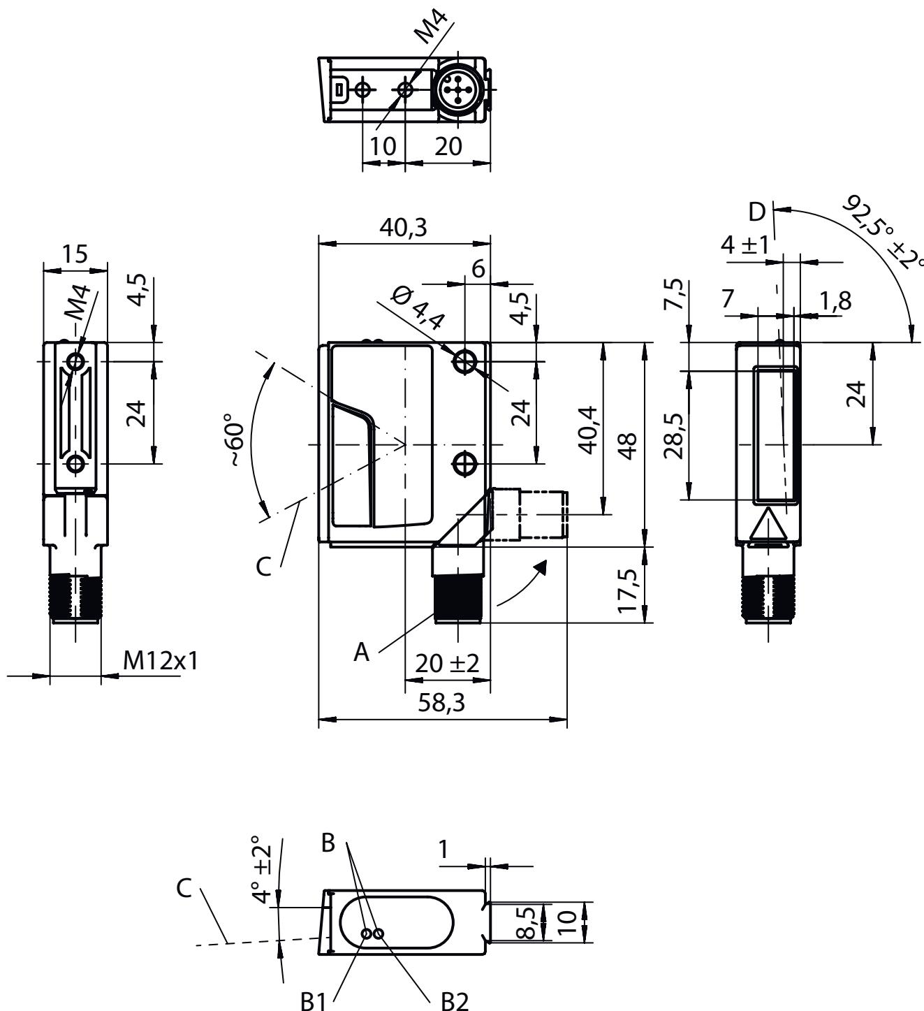
A Turning connector, turnable by 90°
