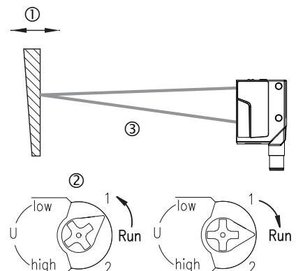
**Reset the analog output to factory settings****Reset 1V/4mA analog output at 25mm:**
