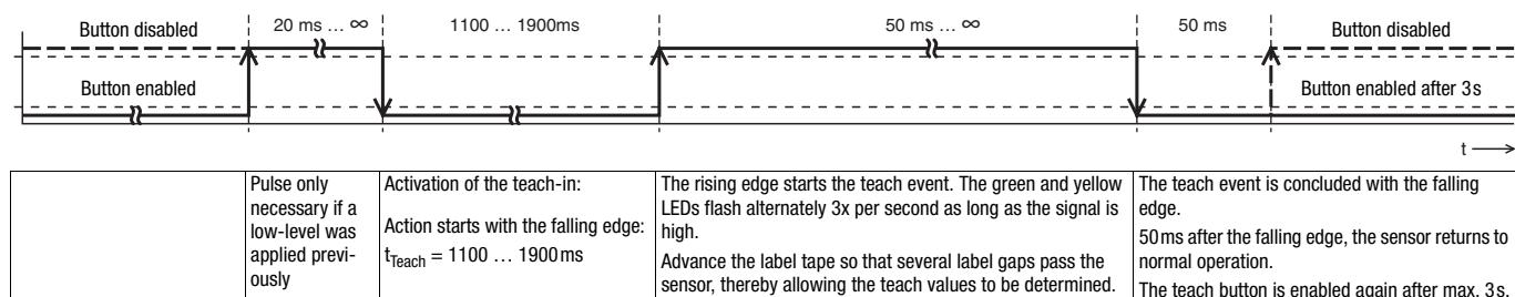
The red LED lights if a teach error occurs (e.g. the label cannot be reliably detected due to insufficient signals).
