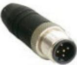
50040099 | TS 01-5-SA  | Terminator plug | Suitable for: DeviceNet, CANopen<br>Function: Bus termination<br>Connection 1: Connector, M12, Axial, Male, A-coded, 5 -pin |
