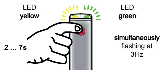
**Adjusting the switching behavior of the switching output – light/dark switching**
