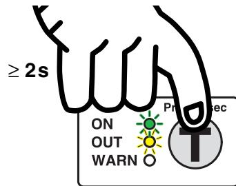
The **green** and the **yellow** LEDs flash **simultaneously** approx.
