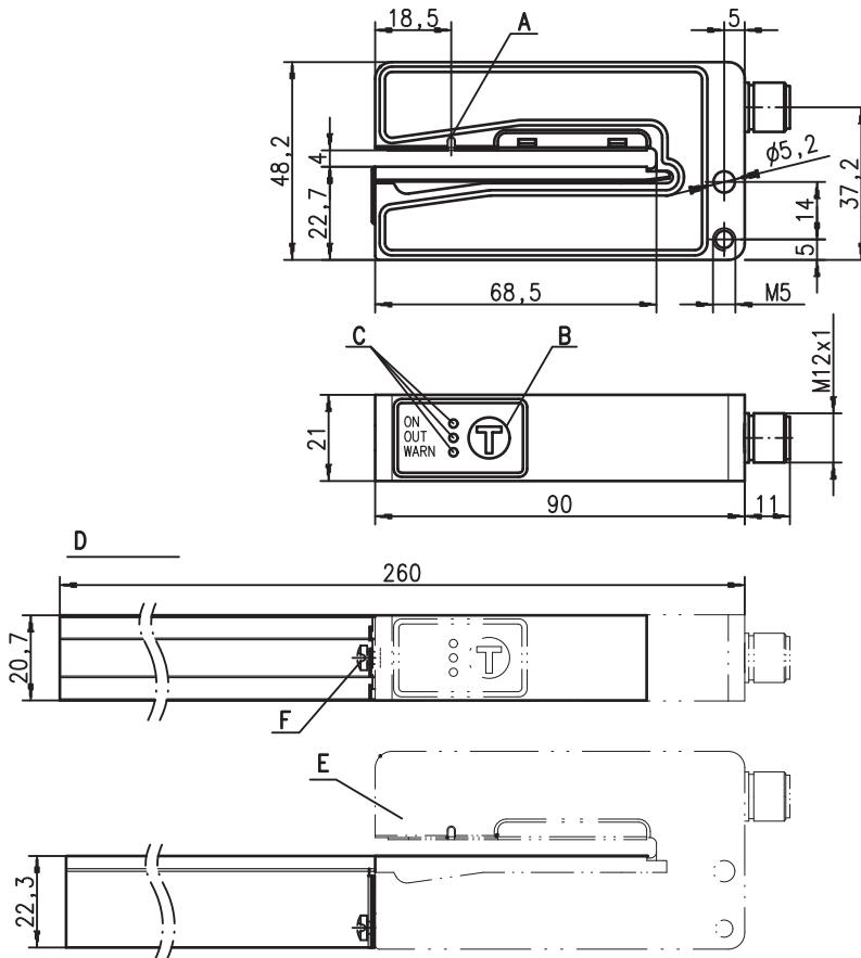
**A** Sensor marker (center of label tape)
