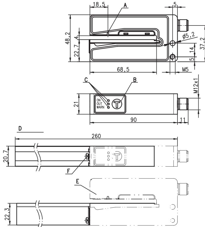
**A** Sensor marker (center of label tape)
