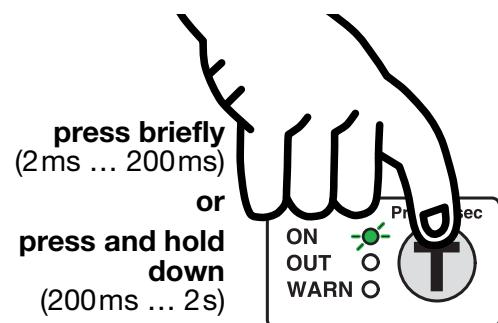
The **green LED** flashes **onetime** quickly or for a longer period time after the button is pressed
