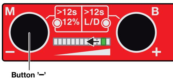
For an optimum setting, the displayed maximum and minimum signal must be symmetric about the switching point (middle of the bar graph).
