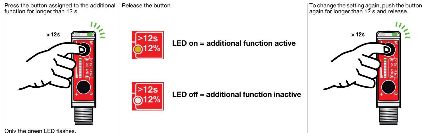
Available special functions (dependent on device model)**12% – switching threshold close to the mark**
