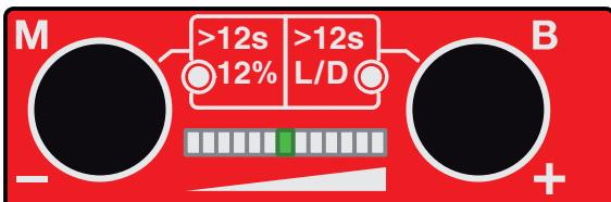
The sensor is set optimally if the maximum and minimum signal are symmetric about the switching point.
