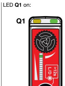
3. Switch between mark and background and watch the bar graph while doing so. Turn the multturn potentiometer until the deflection between the mark and the background is symmetric about the middle of the bar graph.
