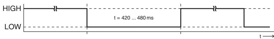
PNP dark switching / dark on, NPN light switching / light on (OUT1)
